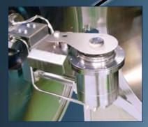
4cm R.F. Ion Source for IBS with Target Indexer
