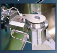
4cm R.F. Ion Source for IBS with Target Indexer
