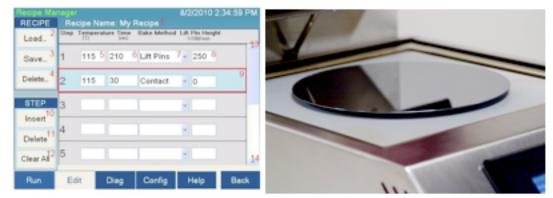
Brewer Science® Cee® equipment engineers have utilized the KLA-Tencor® SensArray measurement probe to measure, track, and record temperature conditions produced by Cee® bake plates. The engineers have meticulously performed these process trials and developed user-friendly temperature matrixes for a variety of common temperatures used for a soft bake (100°C), post-exposure bake (PEB), and post-develop hard bake (205°C) for final curing.
