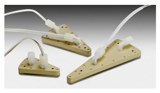
The Dual Zone MegPie is a single-wafer Megasonic transducer for cleaning and sonochemical processing of multiple substrate sizes in one chamber. It applies a uniform dose of acoustic energy to a rotating substrate. The MegPie will improve your process efficiency and lower the process time. It is easy to retrofit to your single substrate processing tool.
