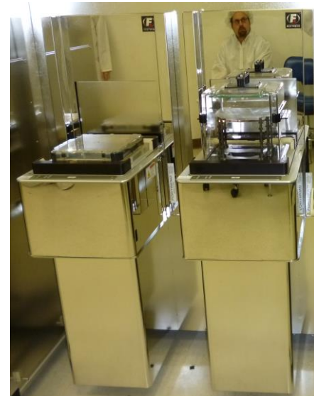
PLM 200Rx on SEMI E63 bolts-M interface load port Adaptor in Reticle Sorter.
