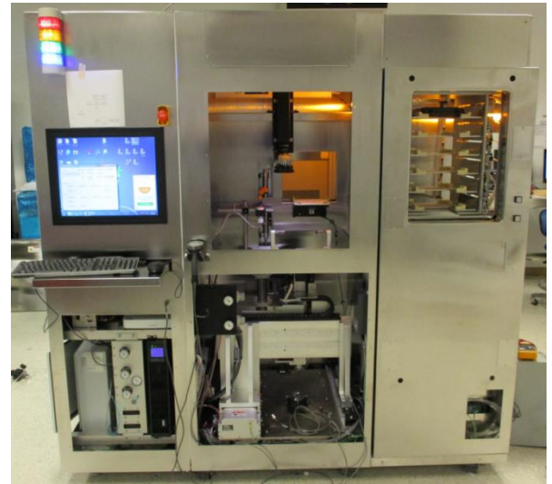
2x RSP 150, DMS Clam shell box with 6 position Auto loader , Bright Light Review module with N2 Blow off, Turn Table with BCR
