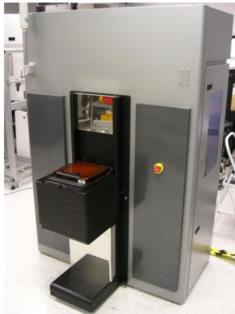
Lamina 201 EFEM for HMI Mask Inspection Tool PLM 200R, Scara Robot, Turn Table, Blank Storage, Bar Code Reader
