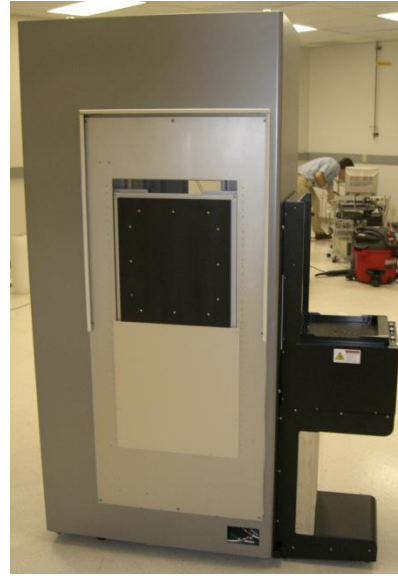
Lamina 201 EFEM for EFEM for Zeiss Merit MG45 Mask repair tool, includes PLM 200R, Scara Robot, Auto process tool chamber opening device and auto door to process tool
